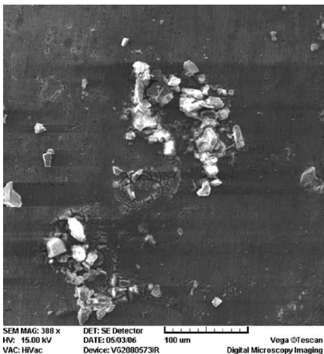
Fig. 9 View of the coming up \text{SiC}_p and clustering phenomenon for the part with dimensions 210 \times 70 \times 40 \text{ mm}^3
