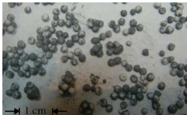
Fig. 3 Pre-puff poly styrene mixed with CMC glue and \text{SiC}_p
